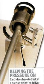
a precise weight to deliver the optimum performance. The counterweight sets the downforce. It's important to get this right, because if it's set too high the sound will be dull and thick in the bass. If it's too low then the sound will become edgy, thin and possibly even distorted
