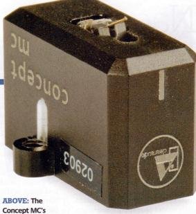
body is in a tough, ceramic-coated aluminium alloy. Clearaudio's choice of a stiff boron rod cantilever is visible here along with its micro line contact stylus and movingcoil generator assembly. Stylus guard is removable and the MC comes in a handsome transparent pyramid case
