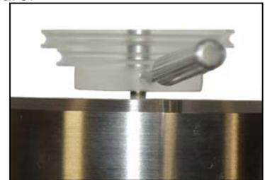
Place the stand alone motor on the top of the motor stand on the position as shown in the right figure. The power switch on the upper side of the motor should show to the outside and the pulley to the turntable platter. The distance between the motor chassis and the turntable platter should be approximately 2 cm (ca. 1/2 inch).
