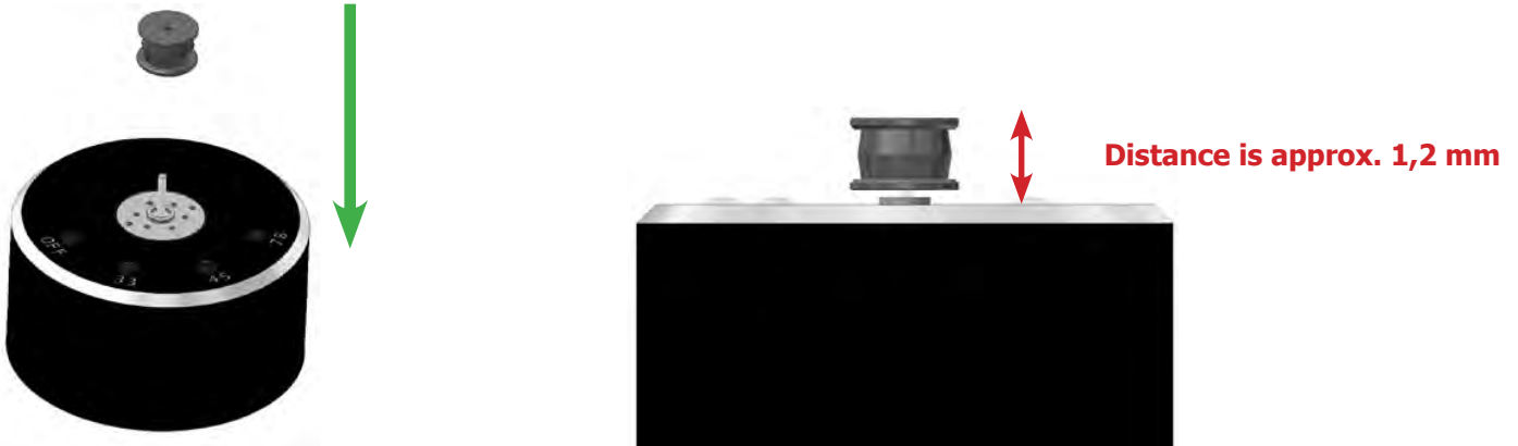
Pic. 10: Setup of the Master Innovation pulley
