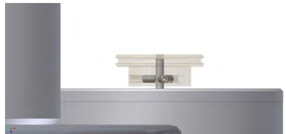
Pic. 21: Setting the motor pulley
