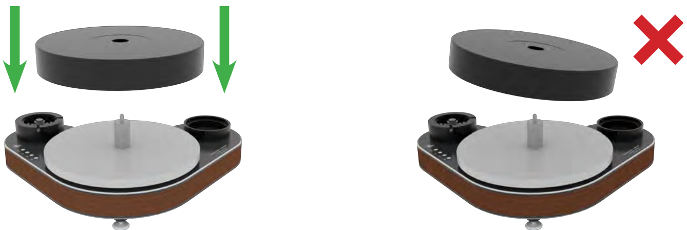
Pic. 10: Mounting the POM platter
