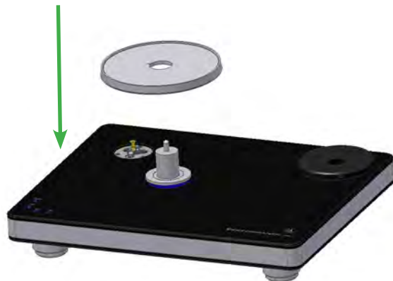
Pic. 7: Setting the sub-platter
