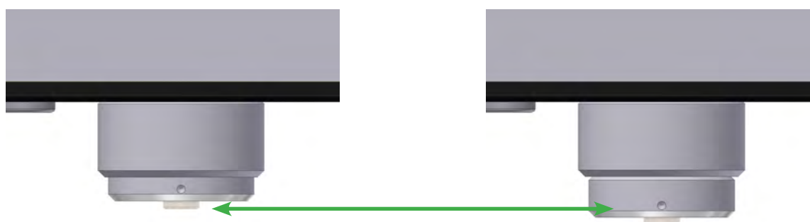
Pic. 9.1: Adjustment of the height
