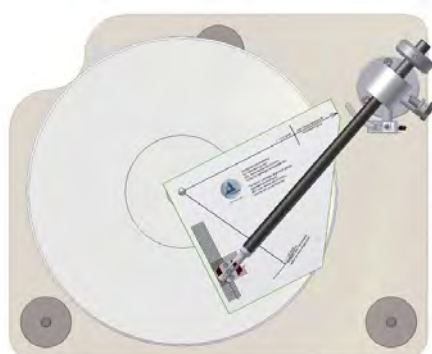
Pic. 10: Alignment of the cartridge
