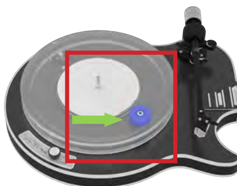
Pic. 8: Levelling the turntable
