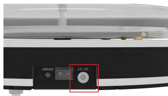
Pic. 10: Power supply of the turntable
