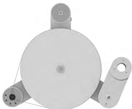
Pic. 6: Rough alignment of the tonearm base
