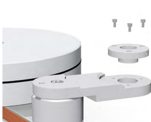
Pic. 5: Mounting the clamping ring
