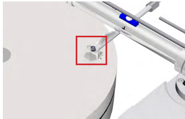
Pic. 18: Adjustment of the azimuth
