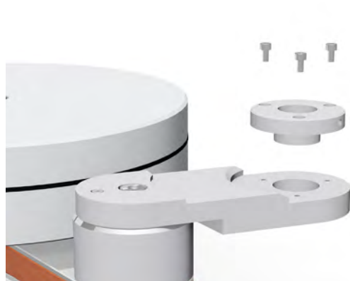
Pic. 5: Mounting the clamping ring
