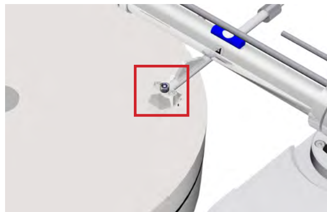
Pic. 18: Adjustment of the azimuth
