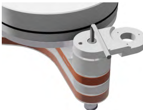
Pic. 10: Mounting of the Unify level base
