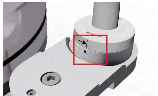
Pic 15b: Mounting direction of the upper part (to the rear)
