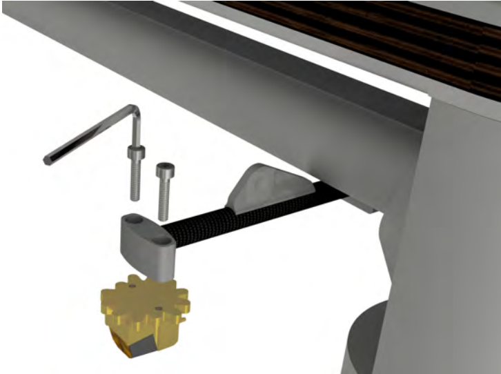
Pic. 15: Mounting of the cartridge
