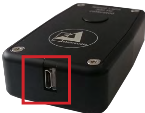
Pic. 1: Micro-USB for continuous current.
