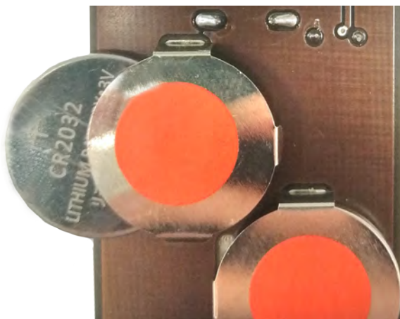
Pic. 5: Inserting the batteries
