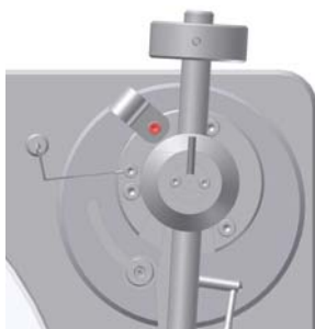
Picture 3: Placing the arm tube to the pivot
