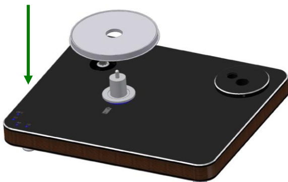
Pic. 5: Seating the sub-platter
