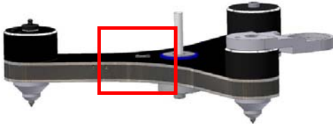
Pic. 5: Removing the lamination
