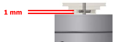
Pic. 13: Mounting the pulley
