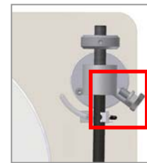
Illustration 3 : Maximum antiskating (Screw is screwed in)
